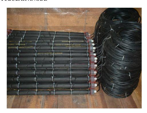
The general working environment for MMO tubular anode in seawater is 600A/m<sup>2</sup>, and in fresh water is 100A/m<sup>2</sup>.
